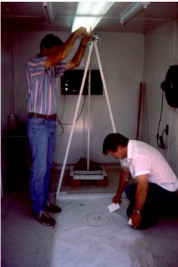
Figure VII.5-2 —Spray tower used to simulate aerially applied sprays for bioassaying grasshoppers in the laboratory. (APHIS photo by Lonnie Black.)
