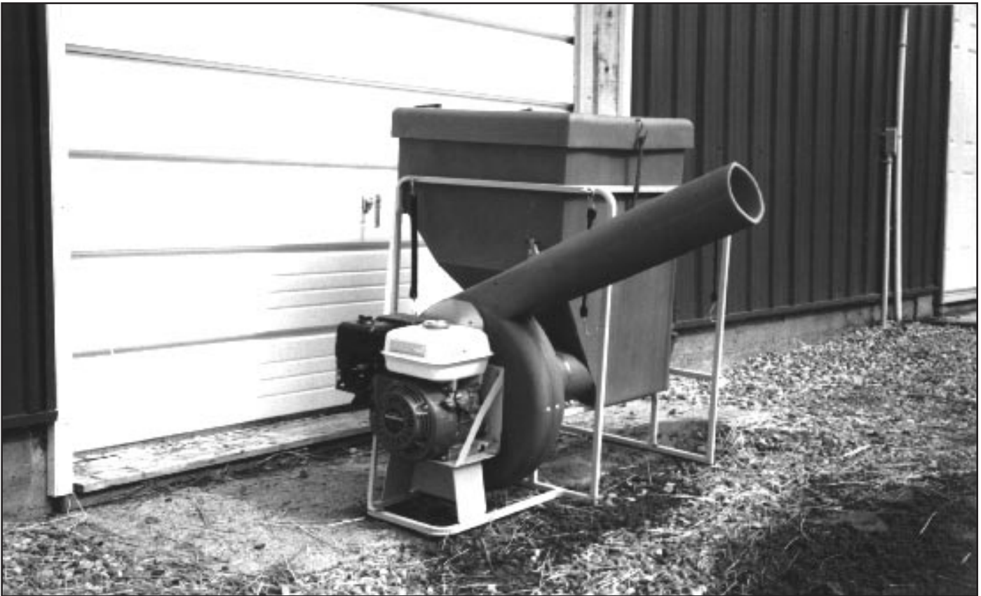
Figure II.19-1 —The Brie-Mar bran spreader fits in the back of a pickup truck and will hold up to 135 lb of bran flakes. This spreader can treat up to a 45-ft swath width. (Photos courtesy of Peacock Industries; used by permission.)
