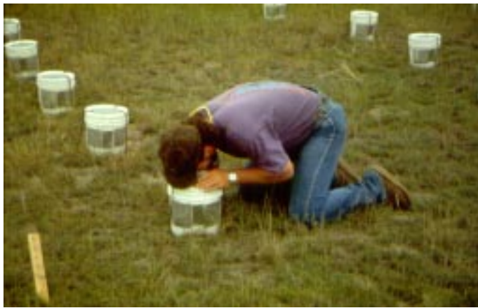
Figure VII.5-7 —Bottomless field cages used to confine test grasshoppers in the field are inspected carefully to determine the daily insect mortality. (APHIS photo by R. Nelson Foster.)
