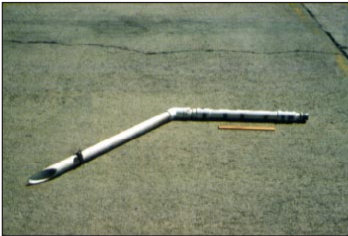
Figure II.18-5 —Ram air tube and air agitation tube before installation on aircraft.
