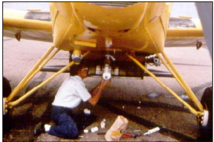
Figure II.18-6 —Front-mounted ram air tube for providing forced air to the air agitation tube during flight.
