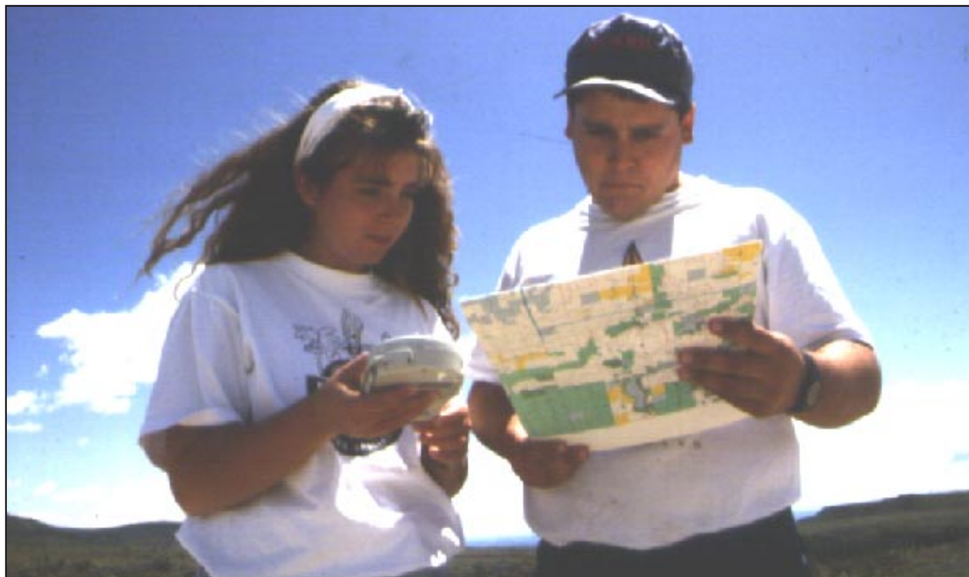
Figure VI.9-1 —One of the newest tools to aid pest managers is a hand-held Global Positioning System (GPS) instrument. GPS provides accurate latitude and longitude coordinates, aiding the process of mapping locations of grasshopper populations. (APHIS photo by Mike Sampson.)
